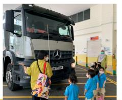
The children watched and learnt the process of latching the bin onto the Rear End Loader, lifting the bin to tip the rubbish in and compacting and moving the rubbish into the body of the truck.
